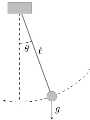
Figure 1: Finding the formula for time period of a pendulum.
