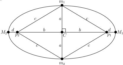
When drawing an oval first set up the material by drawing a line down the middle lengthwise and by marking the centre on that line. From there each pin must be set into the surface of the material on each side of the centre at a specific distance along the long axis. Each pin should be equidistant from the centre, and the material should be cut slightly larger in length and width than the desired size of the oval. The pins cannot be set however, until the appropriate calculations are made.
