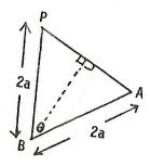
The potential energy of the rod is Wa cos  $\theta$  and that of the other weight  $\frac{1}{2}W \times PA$ . However  $PA = 2(2a \sin \theta/2)$ , so the total potential energy is
