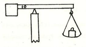
length of material attached at one end to a heavy block. At the other end is a scale pan suspended from a cuphook. A mark labelled 0 is placed on the rod at the balance point when there is no weight on the
