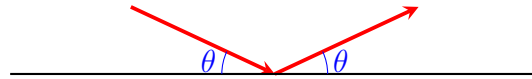
Figure 1: A particle reflecting off a line with the angle of incidence equal to the angle of reflection.
